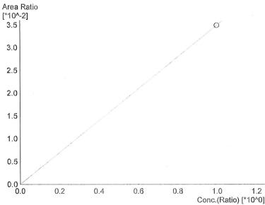
Name: Methanol Detector Name: FID1 Function : f(x)=0.0349393\*x+0 R^2 value= 1.000000 FitType: Linear ZeroThrough: Not Through
