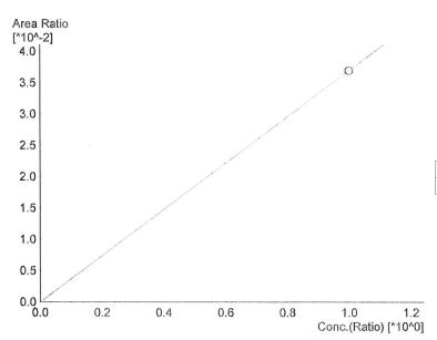
Name: Methanol Detector Name: FID2 Function: f(x)=0.0369243\*x+0 R^2 value= 1.000000 FitType: Linear ZeroThrough: Not Through
