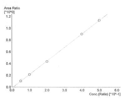
Name: Ethanol Detector Name: FID2 Function: f(x)=2.29738\*x-0.0157435 R^2 value= 0.9998668 FitType: Linear ZeroThrough: Not Through
