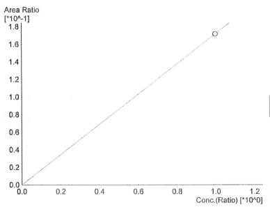
Name: Isopropyl Alcohol Detector Name: FID2 Function: f(x)=0.171759\*x+0 R^2 value= 1.000000 FitType: Linear ZeroThrough: Not Through
